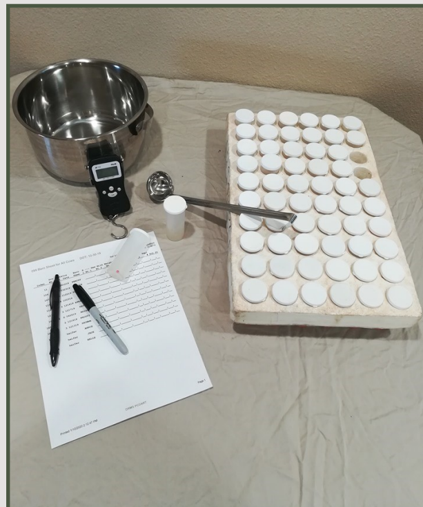
Milk test requires a stainless steel bucket, stainless steel ladle, a certified scale, paper, pencil, and test vials from the lab. A measuring stick and registration papers are needed to verify height and tattoos.
